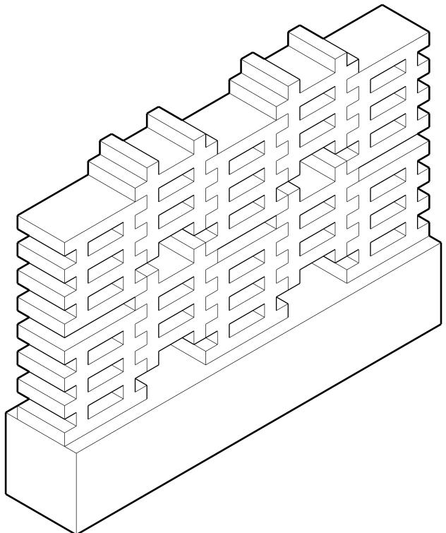
This stacking method strides away from the typical stack. Using our comcept of the puzzle pieces, we have moved various pieces up to create a staggered pattern. In order yo make this stacking method work, corners would need to be added to the ends so that they can be suported.
