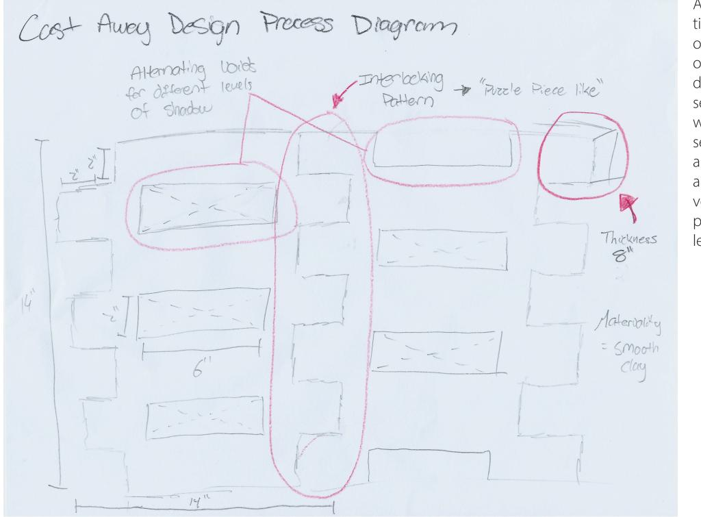
After analyzing our inspiration for the assingmnment, our group decided make our own version. In the process diagram illustrated, you can see that we decided to go with a simple design that resembles a puzzle piece with an interlocking pattern. We also incorporated alternating voids within the two differnt pices to allow for different levels of shadow.
